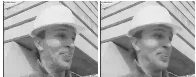
Fig. 17: Performance of the deblocking filter for highly compressed pictures. Left: without deblocking filter, right: with deblocking filter.
